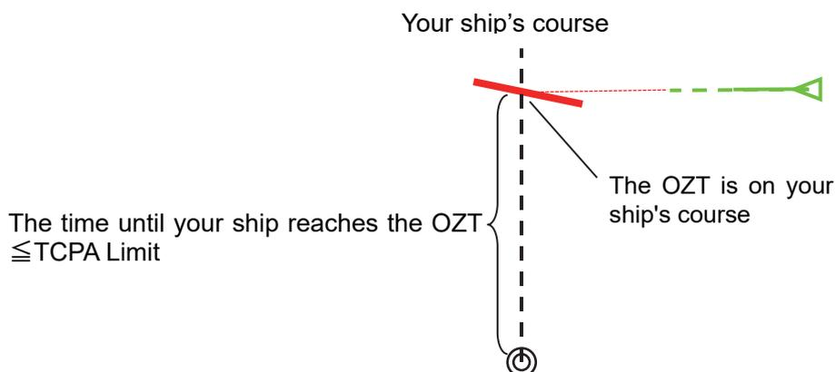
Dangerous OZT is flashing red and an audible alarm. Clicking the [ALART ACK] button will stop the flashing and audible alarm, but the OZT will still be displayed in red for the duration of the dangerous situation.
