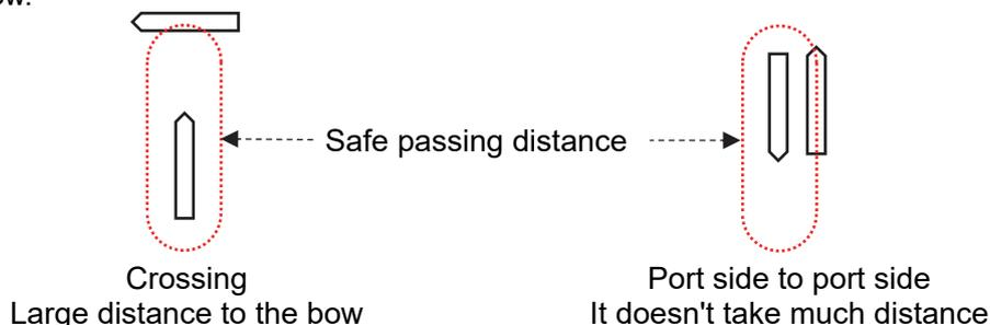
Therefore, by setting the CPA limit to a value smaller than the safe passing distance, it is possible to suppress unwanted CPA / TCPA alarms in congested waters and detect the danger of collision with “Need to Change Course” alarm. See 1.12.9 for details.
