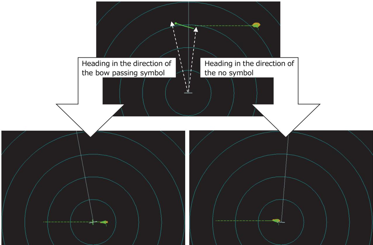
As shown in the figure below, it is possible to display the distance and direction by pointing the cursor over the end point of the OZT.
