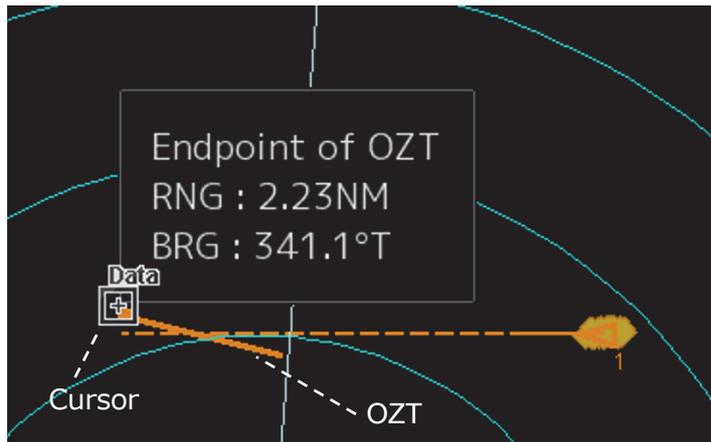
There are multiple targets and you don't sure which OZT belongs to which Target, you can change the color of the corresponding symbol and OZT by pointing the cursor over the OZT or AIS/TT symbol as shown in the figure below.
