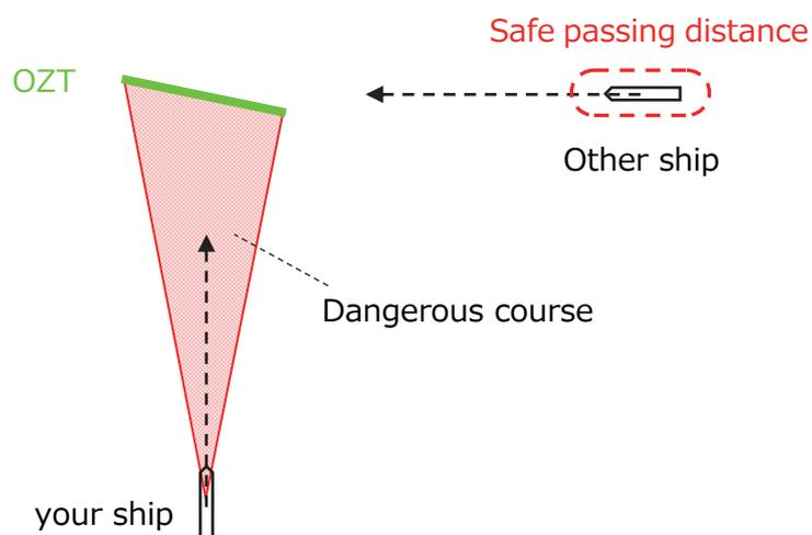
It is also possible to use the OZT as a guide when deciding on a course for avoidance manoeuvre, since avoiding the OZT, as shown in the figure below, allows your ship to maintain a safe passing distance from the other ship.
