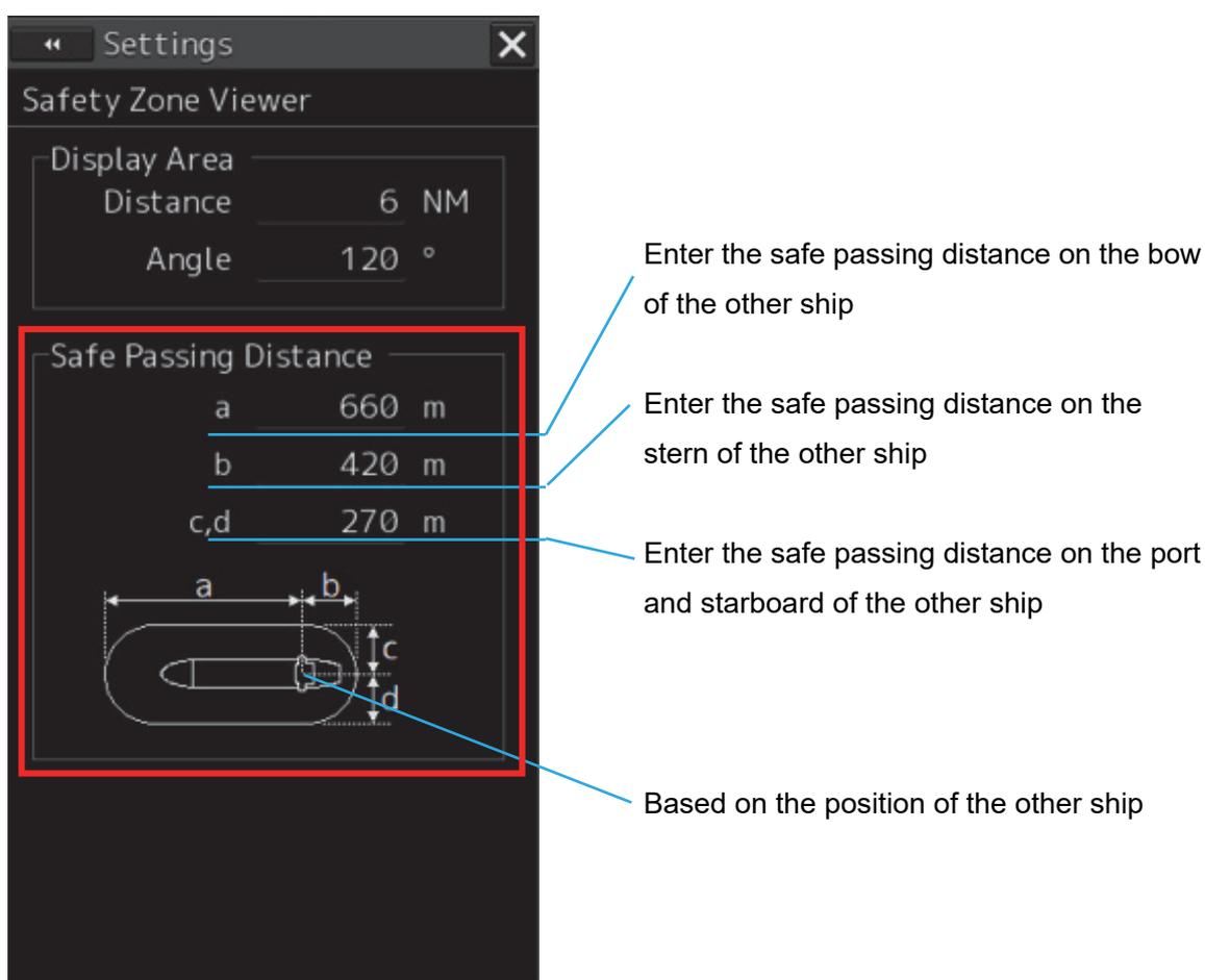
As described in 1.12.3, it is recommended that the CPA limit be smaller than the safe passing distance. Specifically, the CPA limit should be smaller than the smallest of the safe passing distances a, b, c and d. With the default values above, the smallest safe passing distance is 270 m (= 0.15 NM), so it is recommended to set the CPA limit to 0.1 NM.
