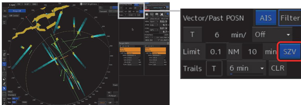
Note: The [OZT] button is disabled when the vector display of TT / AIS is in relative vector mode or when trial maneuver is used. Change the true vector mode and turn off trial maneuver, and then turn on OZT.
