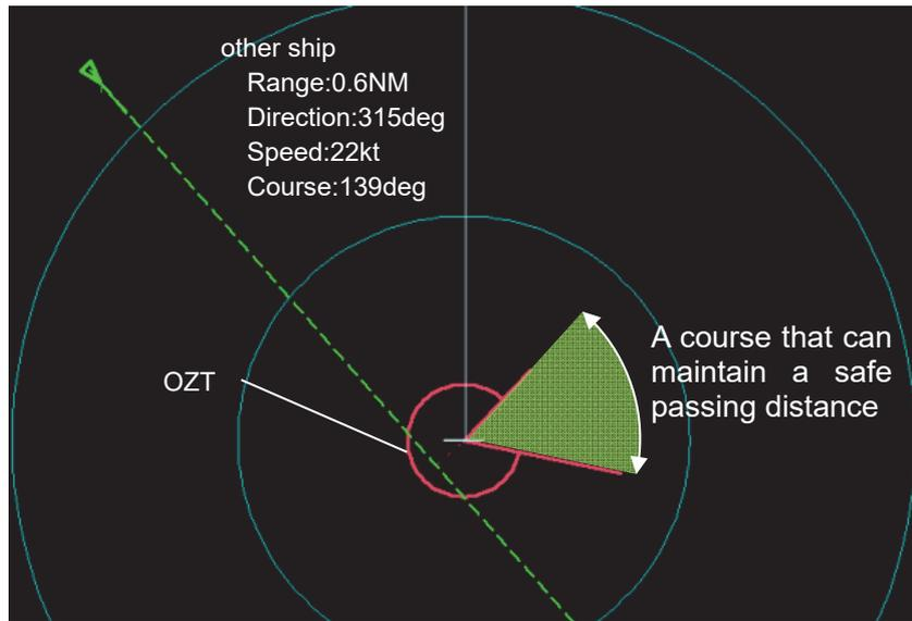
Your ship will not collide with the other ship that is faster than your ship and is moving away from your ship. Therefore, OZT does not exist on such a ship. A ship that does not display OZT can be judged to have a relatively low collision risk.
