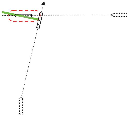
The safe passing distance can be changed in the menu. (Refer to 1.12.9) However, the OZT does not take into account the size of your ship and calculates it based on the ship's CCRP position. If the ship is a large vessel, it is advisable to set a large safe passing distance with a margin or to avoid the other ship so that it is sufficiently far from the OZT.
