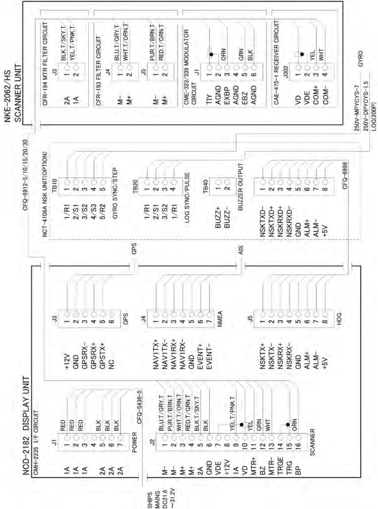
Fig. A15 JMA-3336/HS INTERCONNECTION DIAGRAM
