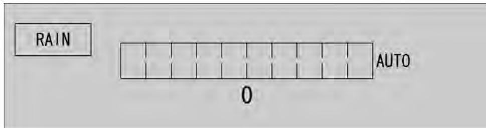
The rain/snow clutter suppression adjustment screen appears when turning the [RAIN] control. Rain/snow clutter suppression can be adjusted between 0 and 100.
