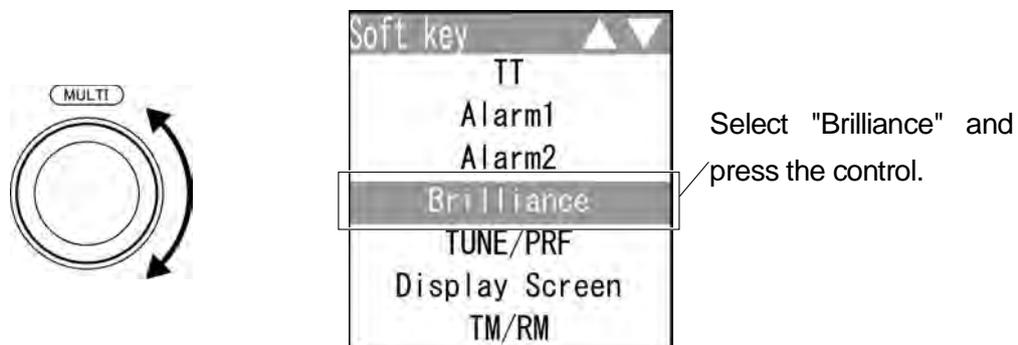
The soft key menu disappears and "Monitor BRILL" of the soft key display is color-inverted.
