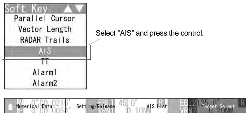
The soft key menu disappears and "Target Select" of the soft key display is color-inverted.
