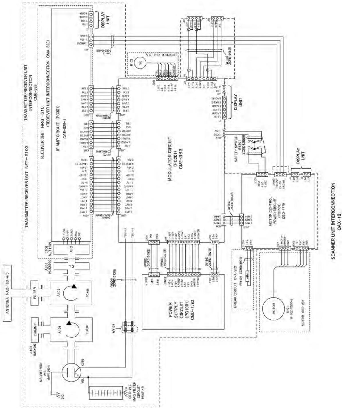
Fig. A10 NCD-2182 DISPLAY UNIT INTERCONNECTION DIAGRAM
