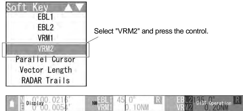
When "VRM1" is selected, the soft key menu is turned off and "DIST Operation" of the soft key display is color-inverted.
