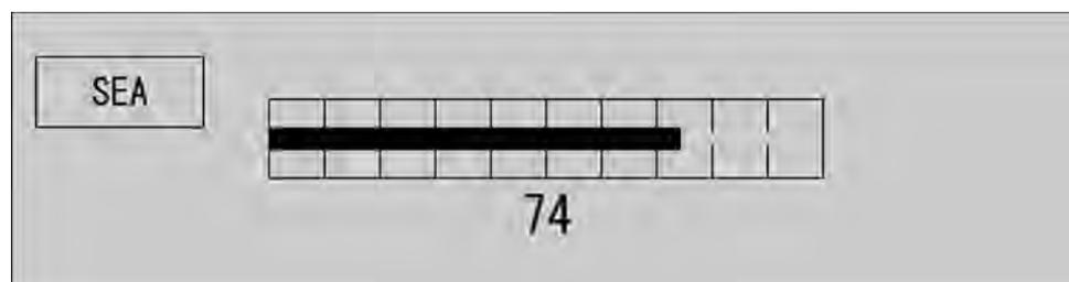
The sea clutter suppression adjustment screen appears when turning the [SEA] control.
