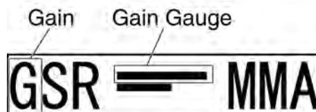
When turning the [GAIN] control, the gain control indication is stretched or shrunk.
