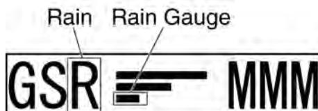
When turning the [RAIN] control, the rain/snow clutter control indication is stretched or shrunk.
