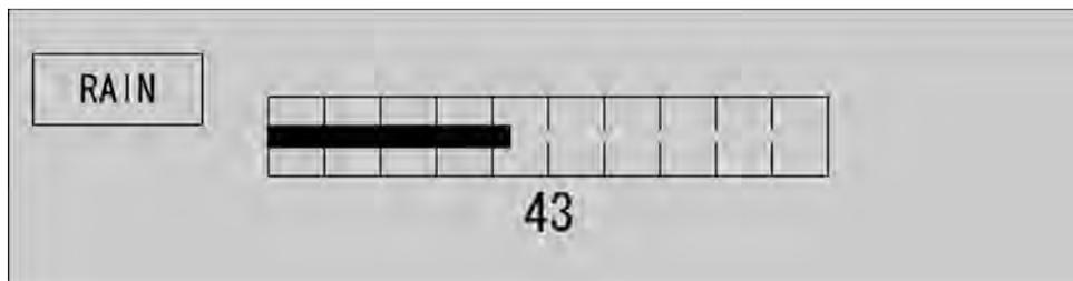
The rain/snow clutter suppression adjustment screen appears when turning the [RAIN] control.
